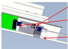
There is a RJ45 contact to the IEX (Can bus) available on the Bottom side of the MP serial.
